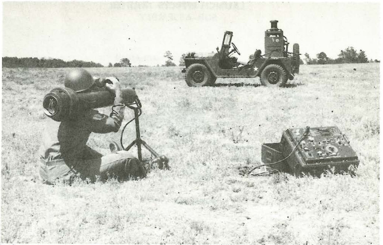
Figure 2. Dragon Training Equipment with Infrared Transmitter Mounted on Jeep
